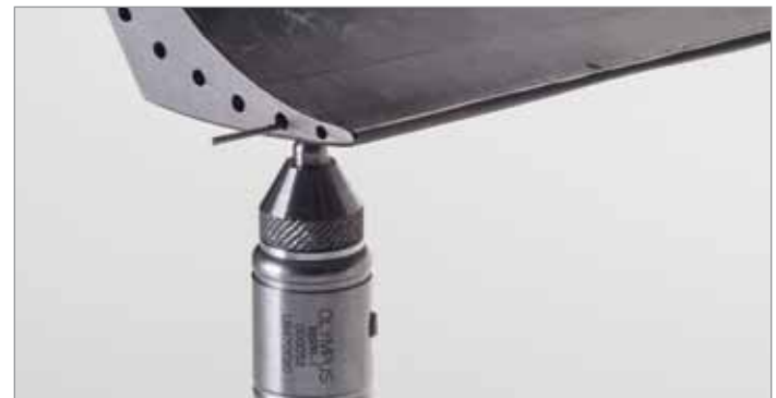
Measurement of a turbine blade using the wire target
