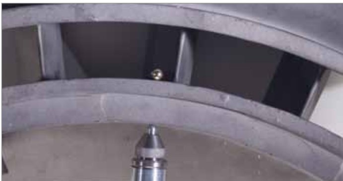
Measurement of a 24.1 mm (0.950 in.) aerospace casting
