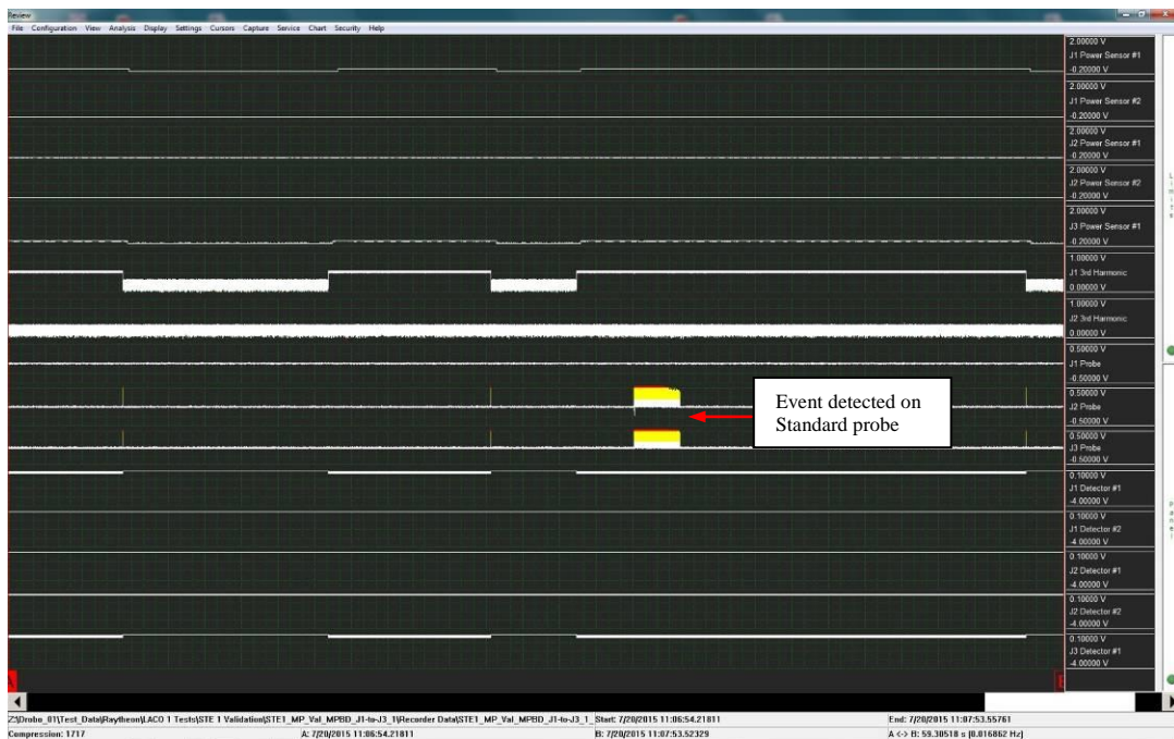
Fig. 6. Multipaction test on standard showing event at 600 Watts peak
