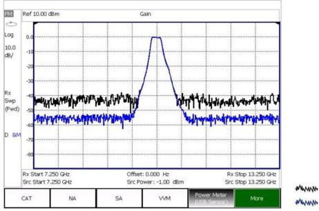
Masured using U2021XA power sensor Manne Measured using U2002A power sensor
