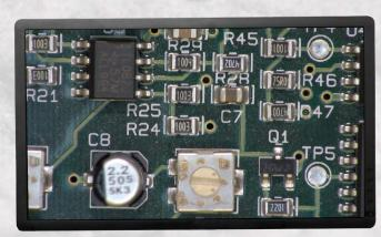
Ideal for inspection of bare solder boards, connectors or assembled boards during SMT-processes. Detect cracks in soldering, spot solder on components, dewetting or bridging in small components. Facilitate your hand soldering of very fine pitch electronic components.
