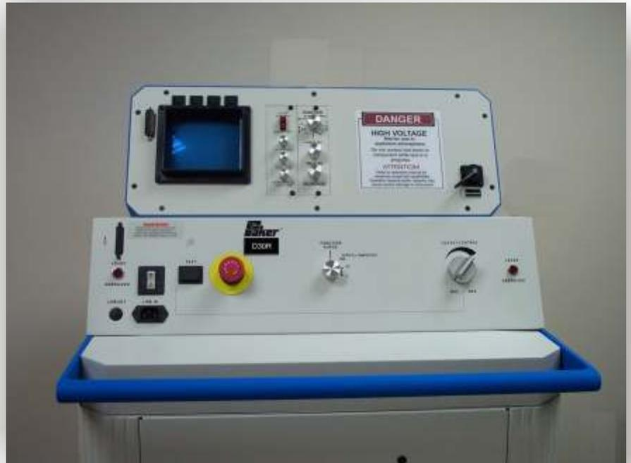
The D30R brings you the latest innovations in the testing of electrical insulation systems. This tester features the proven accuracy and reliability of over 40 years of experience. Specifically designed for shop performance, this digital instrument provides a cost effective solution to large motor testing. The D30R represents Baker Instrument Company's on-going commitment to quality in the design of high performance test equipment.
