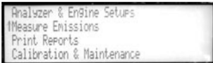
From the Main Menu, use the SELECT buttons to move the arrow up to Analyzer & Engine Setups then press the NEXT button. The following screen will appear.
