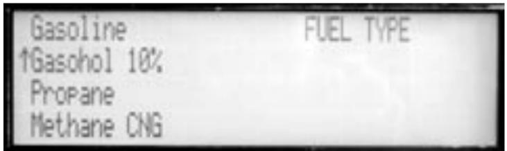
Use the SELECT button to select the fuel type used in the engine, then press the NEXT button. You will be returned to the analyzer setup screen. Selecting the proper fuel will ensure that the CO<sub>2</sub>, AFR, and Lambda measurements are calculated properly.
