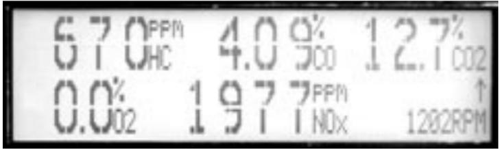
Press either the Up or Down select buttons to alternate between the composite, Grams per Mile and Big Digit screens. The big digit screen displays the five gases and RPM in a large format. Press the NEXT button to go to the main selection screen.
