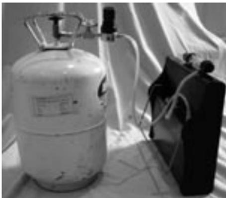
The analyzer will zero the gas bench then ask you to turn on the gas valve on and adjust the pressure regulator until the bar graph is between the two arrows.
