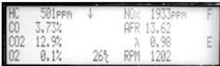
The composite screen displays all five gases, air fuel ration (AFR), Lambda ( $\lambda$ ), and RPM. The screen also shows the status of the memory used during the record functions. Press the NEXT button to go to the main selection screen.
