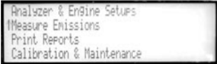
Use the SELECT button to select which analyzer setup you wish to change, then press the NEXT button. Select EXIT to return to the Setup Choices Screen.
