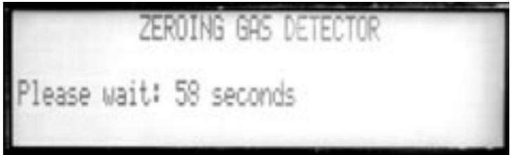
When you select Zero, the analyzer will stop sampling gas from the sample hose and will perform a zero of the bench. There is no need to remove the sample hose from the tailpipe. Zeroing the analyzer periodically will maintain the accuracy of the unit during testing.
