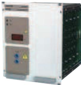
Enables resistors to be added to the high-energy pulse generator type NSG 5000A to modify the generator's impedance. Impedances of  $0.5\Omega$  to  $10\Omega$ , in steps of  $0.25\Omega$  are selectable under software control. The INA 5025 can be operated in either the NSG 5000 basic system chassis, the expansion chassis type INA 5000 or in a special housing type INA 5026.
