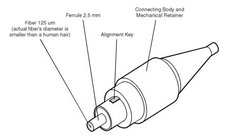
Figure 1-1. Basic components of a connector.
