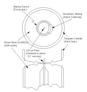
Figure 1-3. Cross-section of the Diamond HMS-10 connector.
