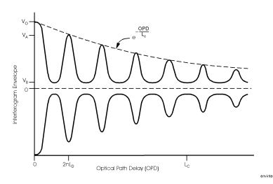
The amplitudes of the peaks decreases exponentially from the largest peak at zero path delay. The exponential decay constant is defined as the coherence length, Lc. The curve that connects the tops of the envelope peaks is given by the following equation:
