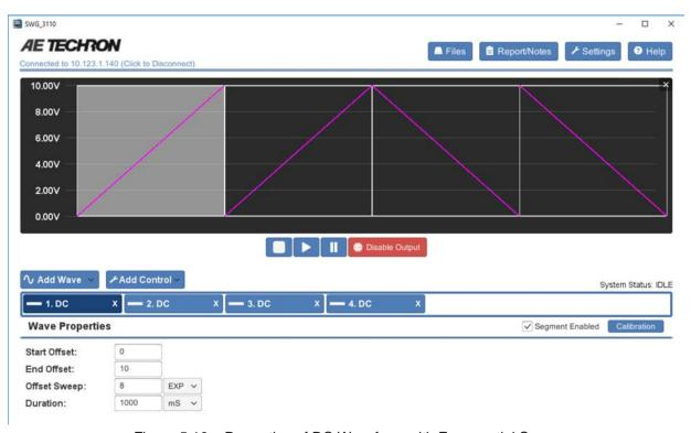
Figure 5.16 – Properties of DC Waveform with Exponential Sweep
