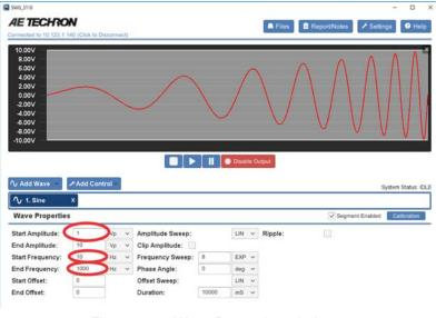
Figure 5.4 – Wave Properties window.
