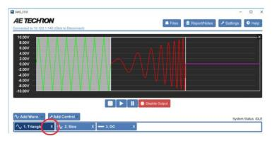
Figure 5.13 – Removing a waveform segment
