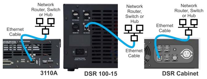
Figure 4.2 - Connecting the 3110A or DSR system to an Ethernet network
