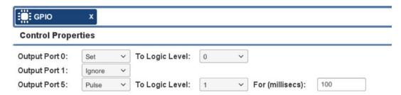
Figure 6.17 – GPIO Output Control Properties
