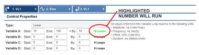
Figure 6.10 - Setting Linear Variable Loop Properties
