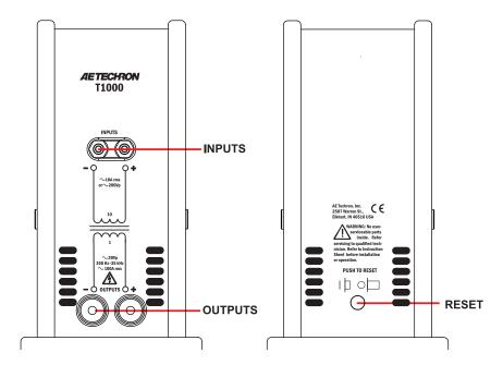
Figure 2 - T1000 Controls and Connectors
