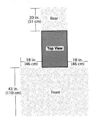
Figure 2.2 – Clearance Recommendations for Cabinet Placement
