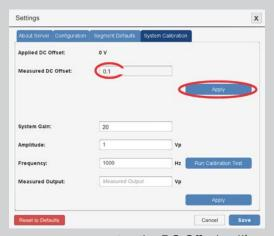
Figure B – Correcting the DC Offset setting.
