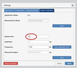
Figure A – Checking the System Gain setting.
