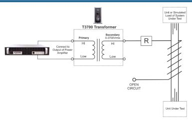
Figure 1 – DO 160 Section 19 Test Load Wiring
