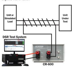
Figure 1 – Test Setup for RTCA DO160 Section 19.3.5 using the CR-600
