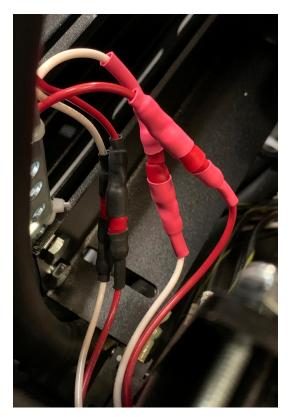
Figure 2.14 – Reconnecting the fan wiring
