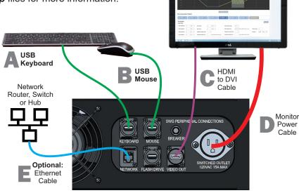
Figure 2.4 - Connecting the 3110A Cables and Accessories on a DSR Series Cabinet
