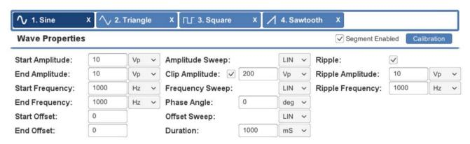
Figure 6.1 – Alternating Waveform Properties (all wave types except Ripple and DC)
