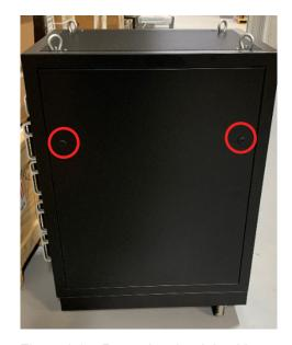
Figure 2.9 – Removing the right side panel
