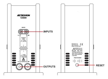
Figure 2 - T2000 Controls and Connectors
