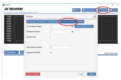
Figure 5.1 – System Calibration tab.
