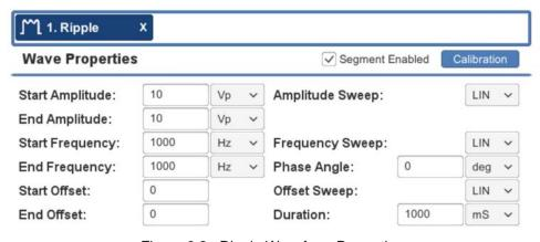
Figure 6.2- Ripple Waveform Properties
