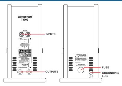
Figure 2 – T3700 Controls and Connectors
