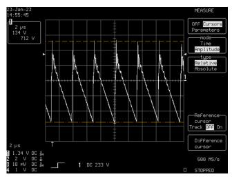
Figure 4 – Example of output from the CR-600 when adjusted for a repetition period of 0.2 to 10 microseconds
