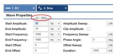
Figure 5.10 – Viewing the allowable range for a waveform property.
