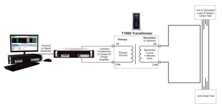
Figure 1 – DO 160 Section 19 Test Load Wiring
