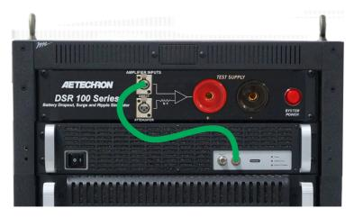
Figure 2.5 – Connecting the 3110A to the Direct Amplifier Input
