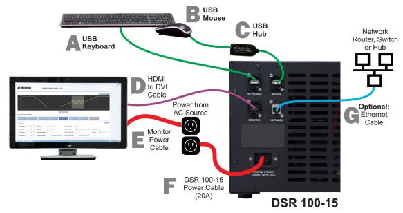
Figure 2.3 - Connecting the 3110A Cables and Accessories on the DSR 100-15/25
