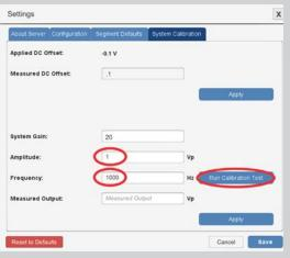
Figure C - Running the Calibration Test.
