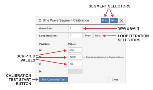
Figure 3.2 – Scriped Variable Loop Calibration Values Window
