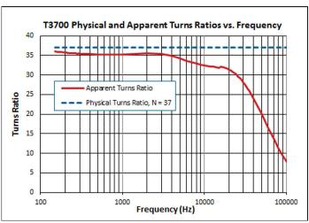
Figure 4- Physical and Apparent Turns Ratios vs. Frequency
