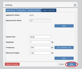
Figure E – Saving the System Calibration Settings
