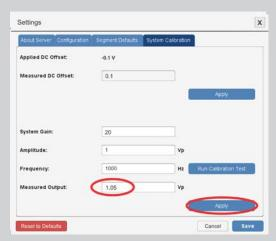
Figure D – Correcting the System Gain setting.
