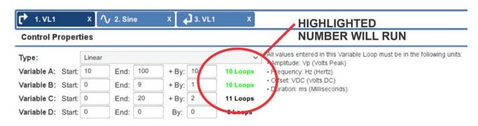
Figure 6.11 – Adding Additional Variables to a Linear Variable Loo
