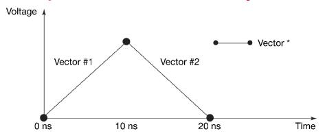
(\*) The waveform is created by specifying multiple vectors (time, voltage). Each vector can be set within the ranges of vector length and voltage.
