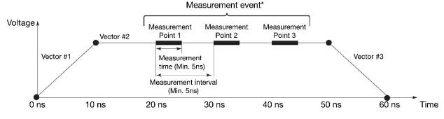
(\*) As well as the measurement event, the range change and trigger event can be specified in the vector.
