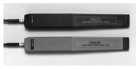
Frequency Range 11940A: 30 MHz–1 GHz 11941A: 9 kHz–30 MHz
