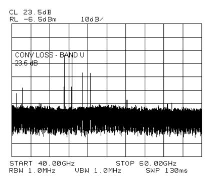
Figure 2-10 Store and correct for conversion loss.
