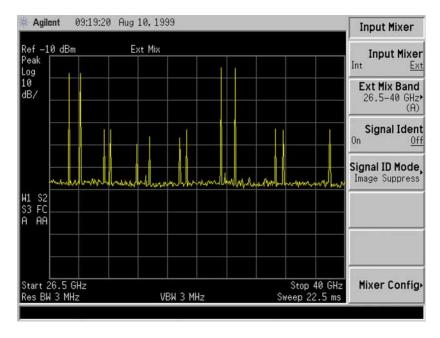
Identification of valid responses is achieved by simply turning on the signal-identification feature. (instrument preset selects the Image Suppress signal identification mode.) Press **Input/Output**, **Input Mixer**, **Signal Ident (On)** and note that now only the valid response (35 GHz) remains.
