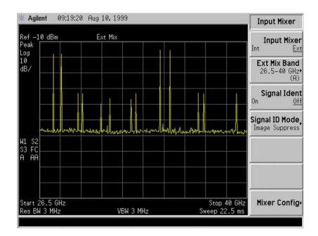
Identification of valid responses is achieved by simply turning on the signal-identification feature. (instrument preset selects the Image Suppress signal identification mode.) Press **Input/Output**, **Input Mixer**, **Signal Ident (On)** and note that now only the valid response (35 GHz) remains.
