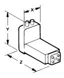
1. Waveguide attachment screws enter blind holes in the flanges of the mixers.
