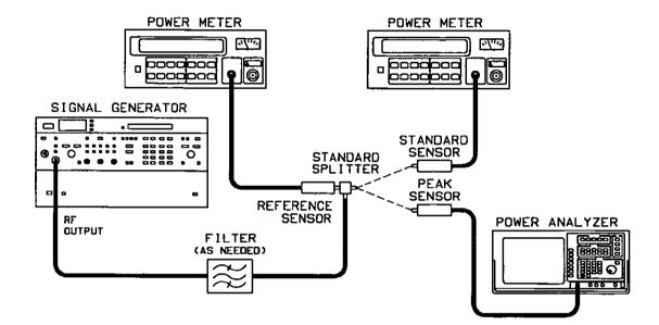
Figure 6-3. Power Level Measurement Setup
