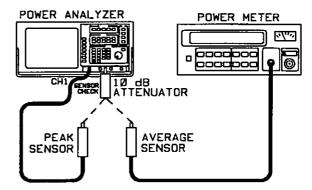
Figure 3-1. SENSOR CHECK Source Check Setup
