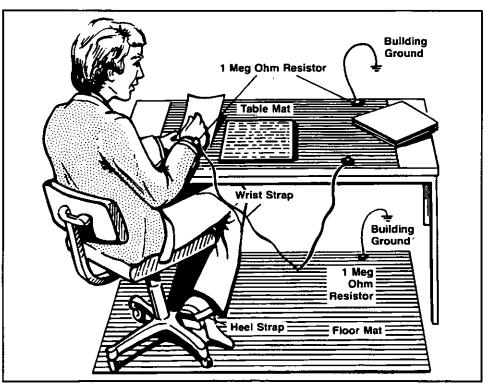
Figure 5-2. Static-Safe Workstation
