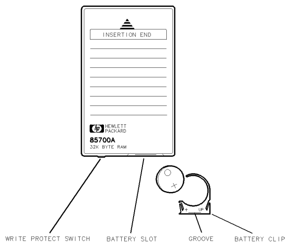
Figure 3-3. Memory card battery replacement.
