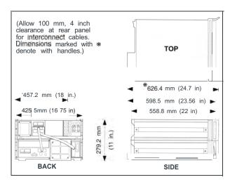
Fig.7. Instrument dimensions with and without handles
