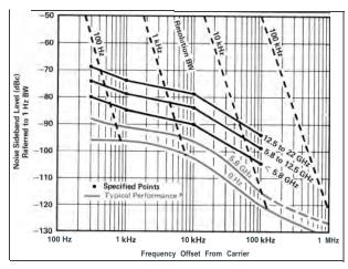
Fig. 2. Single sideband noise normalized to 1 Hz BW vs offset from carrier
