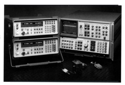
The tracking sources give the HP 8566B dynamic range greater than 125 dB up to 12.5 GHz and greater than 105 dB through 22 GHz.
