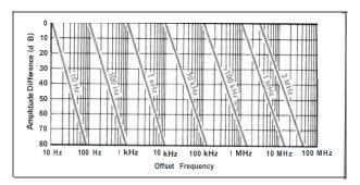
Fig. 1. Typical spectrum analyzer resolution
