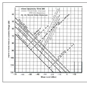
Fig. 4. Typical optimum dynamic range
