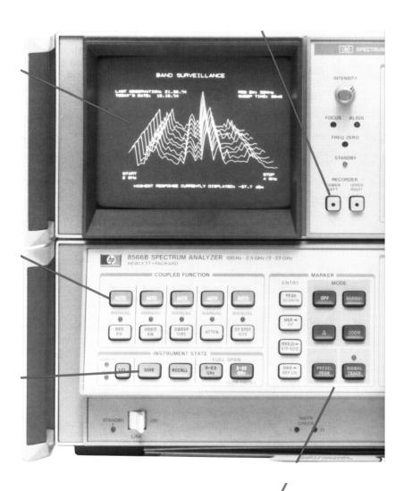
\* Instrument sweeptimes greater than or equal to 20 ms Measurement aids include four tunable markers for direct and relative signal measurements Powerful signal and traceprocessing functions perform complex data analysis
