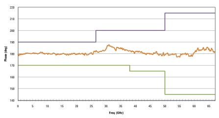
Figure 5. U9391G Comb Generator Phase at 10 MHz PRF
