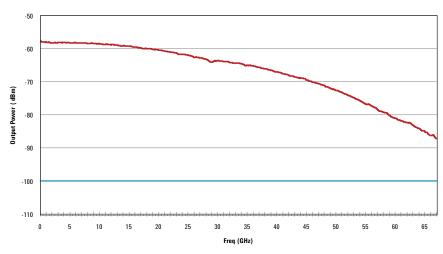
Figure 8. U9391G Comb Generator Output Power at 10 MHz PRF
