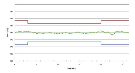
Figure 3. U9391C Comb Generator Phase at 10 MHz PRF
