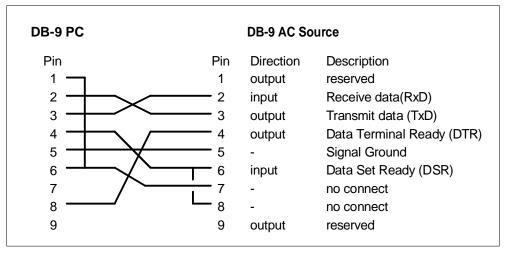
Figure 8-3: RS232C Interface Cable Wiring Diagram
