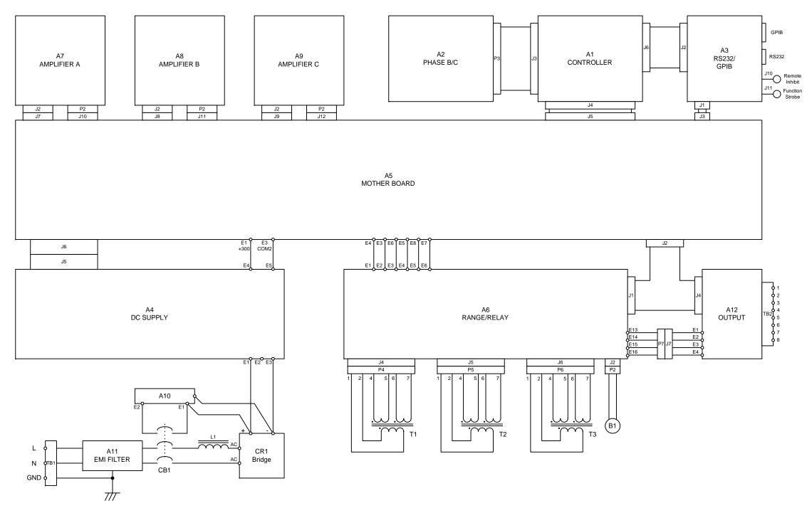
Figure 5-1: AC Power System Block Diagram
