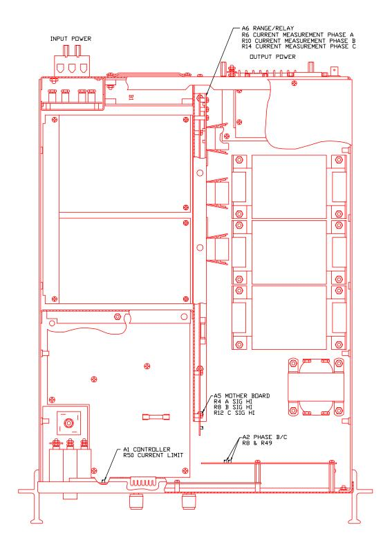
Figure 6-3: Internal Adjustments
