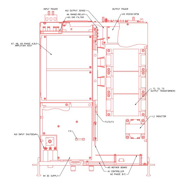
Figure 7-1: Assembly Location
