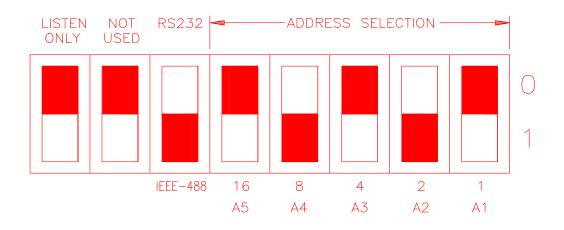
Figure 8-2: GPIB Address Selection Switch
