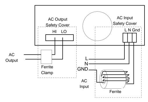
Figure 3-5: Input and Output Wiring
