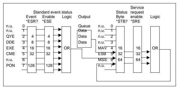
Figure 12-1: AC Source Status System Model
