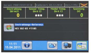
DisplayColor LCD with LED backlightResolution480 x 272 pixelsSuitable for use in sunlight
