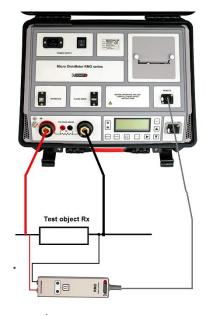
Provided that, for a series of tests, the same test current is fed through the test object, multiple measurements can be carried out with the RMO Remote Control Unit.
