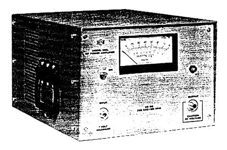
The ENI Model 350L is an all solid state amplifier which has a flat frequency response from 250 kHz to 105 MHz. It provides 50 watts of linear power with low harmonic and intermodulation distortion. Gain is 50 dB nominal, with a variation of less than  $\pm 1.5$  dB over the entire frequency range. Input and output impedance are 50 ohms and the unit may be driven to full power output by most RF synthesizers, signal generators and swept signal sources.
