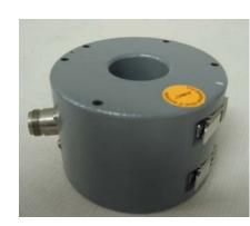
The F-16-1 is used to measure conducted emissions from 10kHz to 50MHz. Its useable frequency range is 10Hz to 70MHz. The basic F-16 probe has a transfer impedance of  $4\Omega$  from 30kHz to 50MHz. The F-16-1 with the power absorbing terminator has a constant transfer impedance of .5 $\Omega$  from 20kHz to 50MHz. All configurations of the F-16 probe can handle 400 amperes of primary power line currents from DC to 60Hz without saturating or impacting the transfer impedance of the probe.
