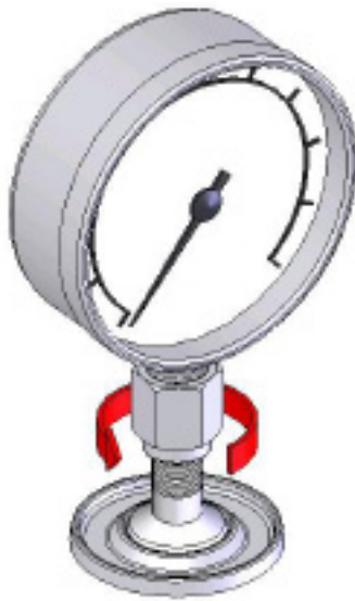
Figure 2-2. Connect Assembly to Test Port
