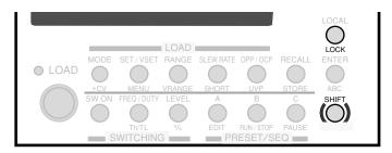
Fig. 5-10 Keys used in the lock function
