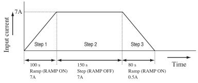
Fig. 6-9 Normal sequence execution example
