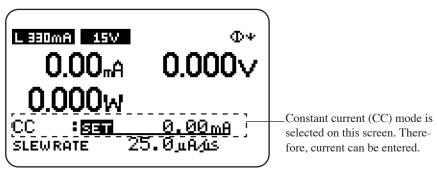
Fig. 2-5 Basic setting entry condition
