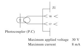
Fig. 6-46 Equivalent output circuit
