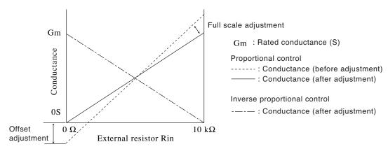
Fig. 6-31 Control the resistance using external resistance
