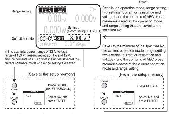
Fig. 6-4 Contents stored to the setup memory
