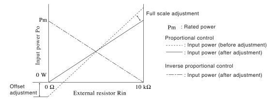
Fig. 6-35 Control the wattage using external resistance
