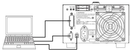
Fig. 1-2 PLZ-4W and PC connection diagram
