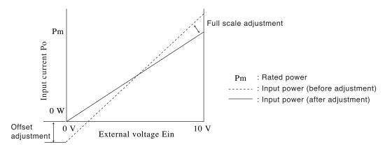
Fig. 6-33 Control the resistance using external voltage
