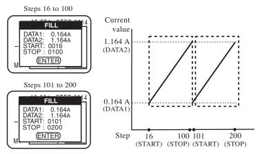
Fig. 6-18 Setup example using the FILL function
