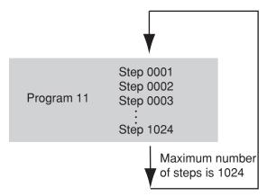
Fig. 6-16 Conceptual diagram of program and step
