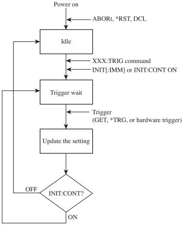
Fig. 7-2 Trigger wait status control using INIT:CONT
