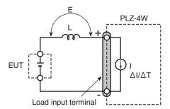
Fig. 2-7 Load wire and inductance
