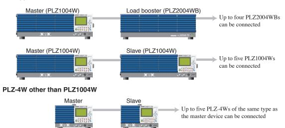
Fig. 1-3 Parallel connection
