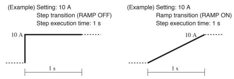
Fig. 6-12 RAMP sequence example
