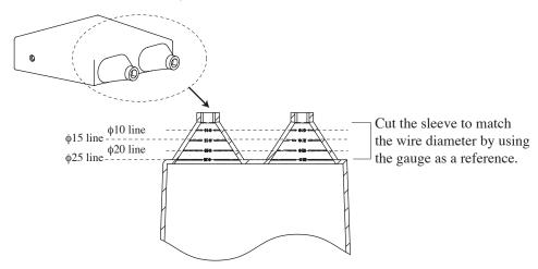
Fig. 2-13 Load input terminal cover
