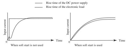
Fig. 5-8 Operation of the soft start function
