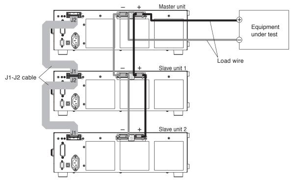
Fig. 6-49 Parallel connection of two slave units
