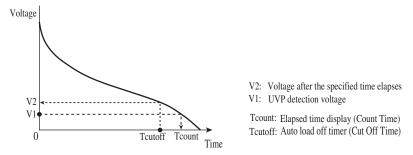
Fig. 6-8 Count Time and Cut Off Time
