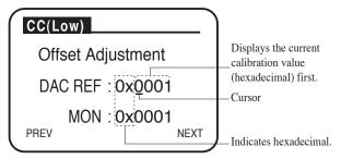
Fig. 8-7 CC (Low) Offset Adjustment screen
