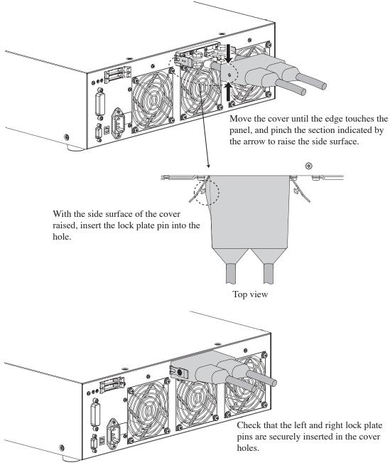
Fig. 2-16 Attachment of the load input terminal cover
