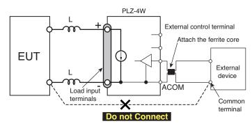
Fig. 6-22 When operation under high-speed load simulations
