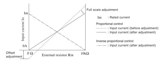
Fig. 6-27 Control the current using external resistance
