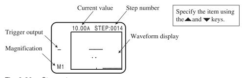
Fig. 6-20 Step setup screen
