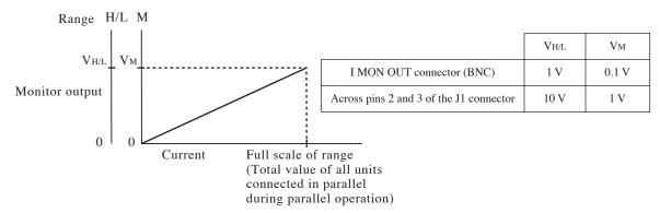
Fig. 6-48 Current monitor output
