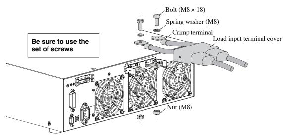
Fig. 2-15 Connection to the load input terminal on the rear panel
