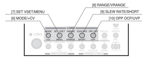
Fig. 4-4 Operation panel (LOAD)
