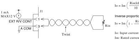
Fig. 6-26 Equivalent circuit
