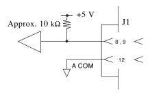
Fig. 6-43 Equivalent input circuit
