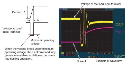
Fig. 2-8 Waveform example: Generate unstable oscillation or hunting operation
