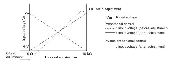
Fig. 6-39 Control the wattage using external resistance
