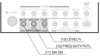
Fig. 4-5 Operation panel (SWITCHING)
