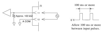
Fig. 6-42 Equivalent input circuit
