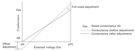
Fig. 6-29 Control the resistance using external voltage
