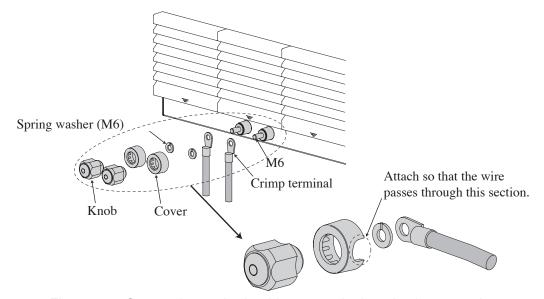
Connection to the load input terminal on the front panel Fig. 2-17
