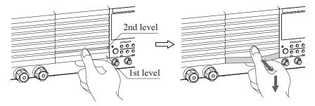
Fig.8-1 Removing the louver
