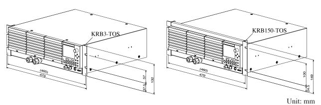
Fig. 1-5 Rack mount bracket
