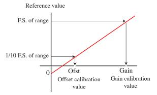
Fig. 8-4 Offset and gain calibration
