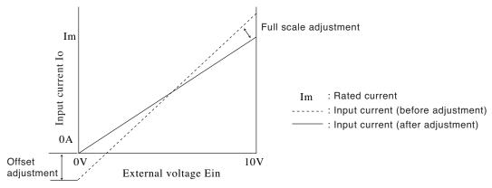
Fig. 6-25 Control the current using external voltage
