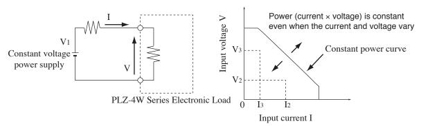
Fig. A-7 Equivalent circuit of the CP mode and operation
