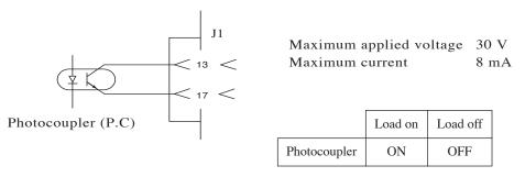
Fig. 6-41 Equivalent output circuit
