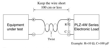
Fig. 2-9 Length of wiring
