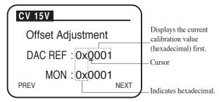
Fig. 8-8 CV 15V Offset Adjustment screen
