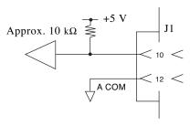
Fig. 6-45 Equivalent input circuit
