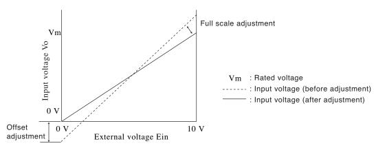
Fig. 6-37 Control the current using external voltage
