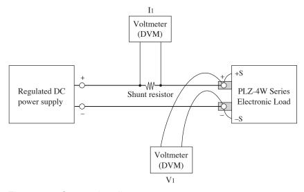
Fig. 8-5 Connection diagram
