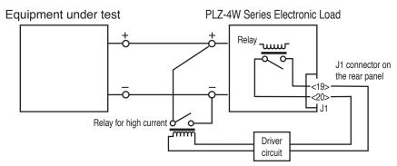
Fig. 5-11 Connection example of a relay for high current
