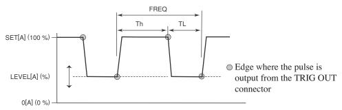
Fig. 6-5 Characteristics diagram of a switching waveform
