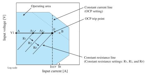
Fig. A-6 Transition of the operating point in CR mode (OCP trip point)
