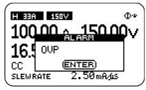
Fig. 2-10 Overvoltage alarm
