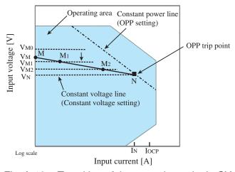
Fig. A-10 Transition of the operating point in CV mode (OPP trip point)
