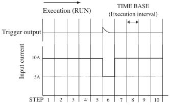
Fig. 6-10 Fast sequence execution example
