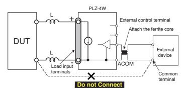
After taking the measure as described herein above, please make sure that the voltage of the load input terminal of the electronic load should not be dropped under the minimum operating voltage and not be exceeded the maximum input voltage.
