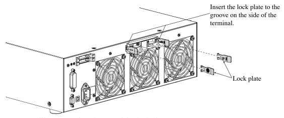
Fig. 2-14 Attachment of the lock plate
