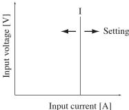
Fig. 3-4 Equivalent circuit of the constant current load and operation
