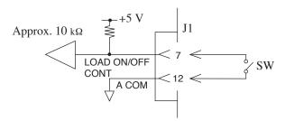
Fig. 6-40 Equivalent input circuit
