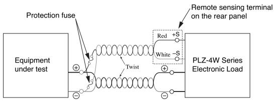
Remote sensing wiring Fig. 6-21
