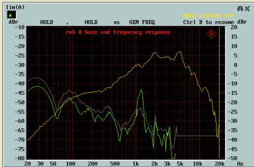
Fig. 14: Frequency response and rub & buzz function for quality assurance in loudspeaker production
