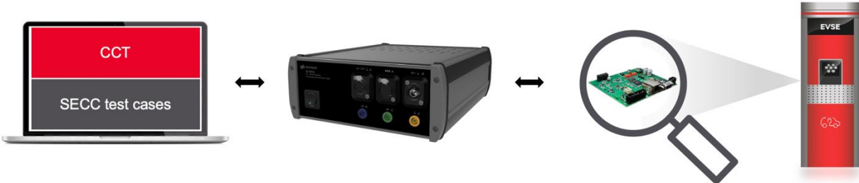
Figure 5. Type approval tests of SECC with Com Tester and CCT
