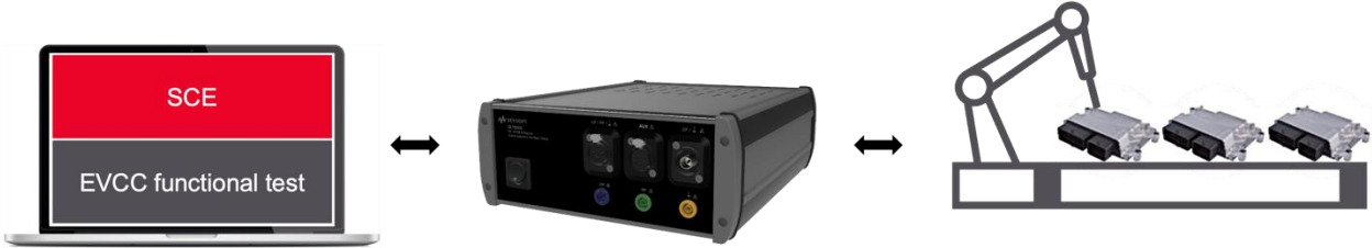
Figure 6. End-of-Line tests of EVCC with Com Tester and SCE
