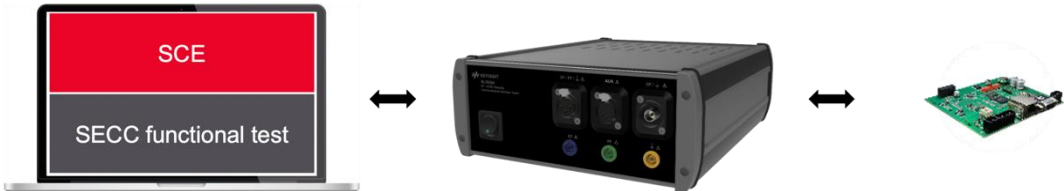
Figure 3. Development tests of SECC with Com Tester and SCE
