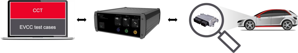
Figure 4. Type approval tests of EVCC with Com Tester and Charging Communication Conformance Test Software (CCT)
