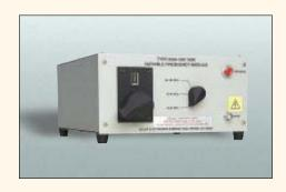
Utilizing the high voltage power source in the **Model 9354-1 Universal Transient Generator**, four individual modules can be connected to provide tuning of damped sine waves from 10 KHz to 50 MHz. A fifth module is available which, when used in conjunction with the **Model 9354-1**, provides 20% frequency steps from 30 MHz to 100 MHz.
