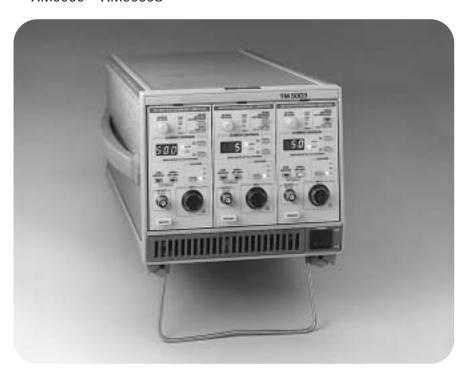
AM5030. Three AM5030s in a TM5003 mainframe. All current measurement parameters can be set using a GPIB controller.
