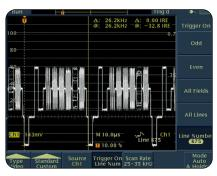
Custom video trigger allows the TDS3000B to trigger on standards such as RS343 (26.6 kHz scan rate).
