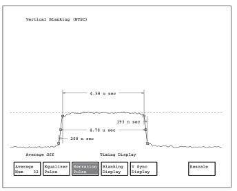
Vertical Blanking Serration Pulse measurement.
