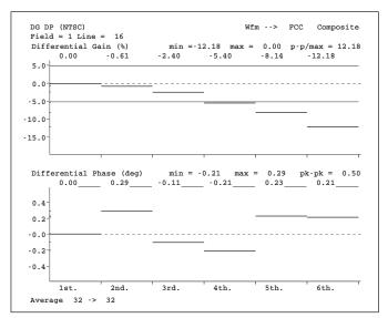
Differential Gain and Phase measurement.
