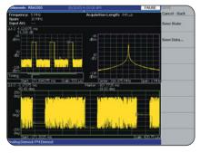
Time-correlated multi-domain view provides a new level of insight about design or operational problems and possible solutions. This example includes frequency, time, and modulation domain views of an AM-modulated pulsed signal with pulseto-pulse phase variation measured in the modulation domain.
