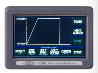
The 4700 Chart Mode automatically provides a scaled graphic presentation of up to 300 readings to aid in verification of voltage ramp and dwell times, undershoot, overshoot and drift.
