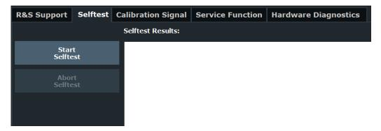
Once the self-test is started, all modules are checked consecutively and the test result is displayed. You can abort a running test.
