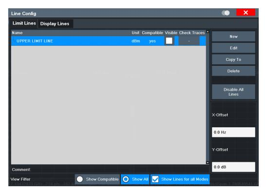
For the limit line overview, the R&S EPL1000 searches for all stored limit lines with the file extension .LIN in the limits subfolder of the main installation folder. The overview allows you to determine which limit lines are available and can be used for the current measurement.
