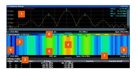
Figure 11-3: Screen layout of the spectrogram result display
