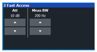
The advantage of the fast access panel is that it is easier and faster to change various settings in a single panel without having to find and access dialog boxes or softkey menus first. In addition, you can still view results while changing parameters, without dialog boxes blocking the view.
