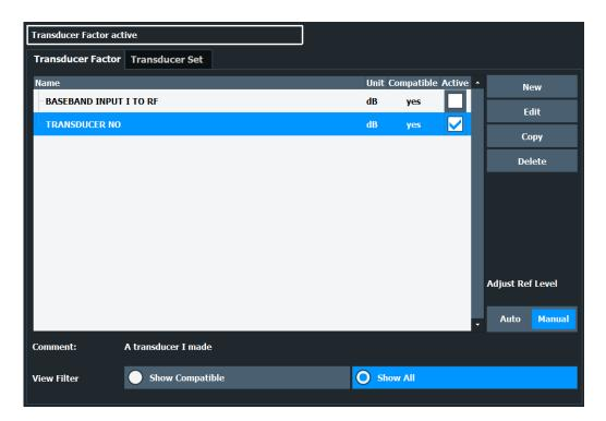
The dialog box contains several tabs, including one to configure transducer factors and one to configure transducer sets.
