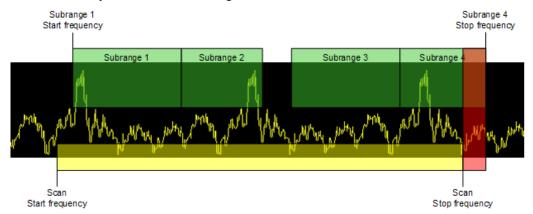
Figure 9-9: Scan range vs subranges of a scan
