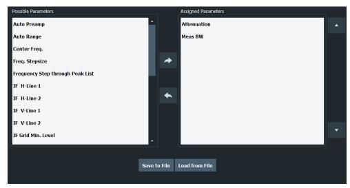
2. To assign an additional function to the panel, select one of the parameters in the left menu and move it to the right menu with the right arrow key (►). Alternatively, you can move items via drag & drop.
