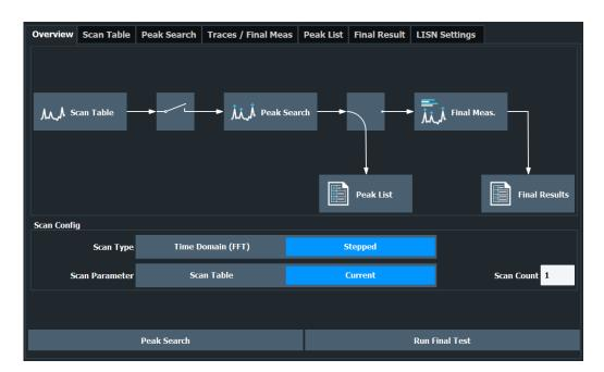
Figure 9-8: Overview of the test automation process
