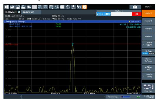
Figure 11-9: Example for an upper limit line
