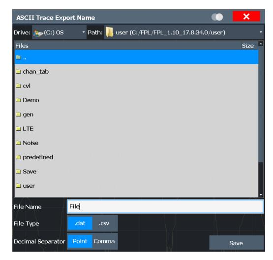
If the spectrogram display is selected when you perform this function, the entire histogram buffer with all frames is exported to a file. The data for a particular frame begins with information about the frame number and the time that frame was recorded. For large history buffers the export operation can take some time.
