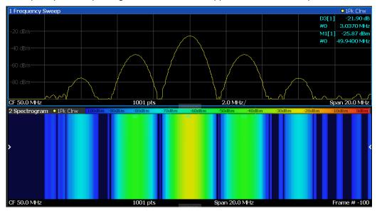
In this example, you see the spectrogram for the calibration signal of the R&S EPL1000, compared to the standard spectrum display. Since the signal does not change over time, the color of the frequency levels does not change over time, i.e. vertically. The legend above the spectrogram display describes the power levels the colors represent.
