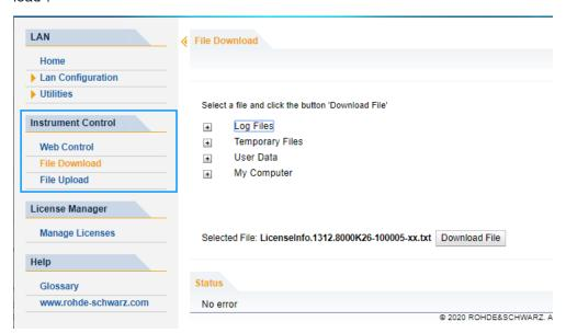
The most commonly used folders on the instrument are displayed. For example, folders that contain user data. From the top-most folder, My Computer, you can access all other folders on the instrument.
