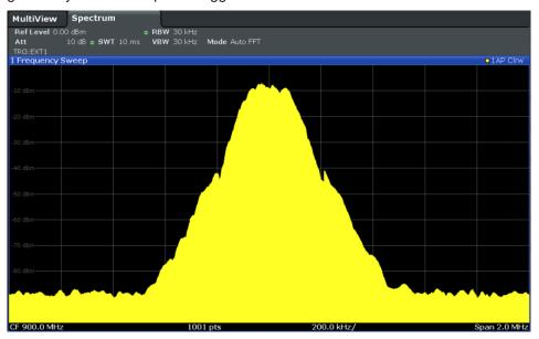
Figure 10-6: GSM signal with GATE OFF
