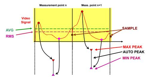
The detectors of the R&S EPL1000 are implemented as digital devices. All detectors work in parallel in the background, which means that the measurement speed is independent of the detector combination used for different traces.
