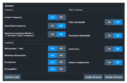
When you couple a parameter across all active measurement channels, a change in the currently selected application is passed on to all other active measurement channels.
