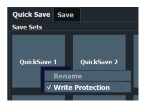
During recall, save sets of type "Instrument" replace the settings of the entire instrument. All other save sets start a new channel setup with the stored settings.
