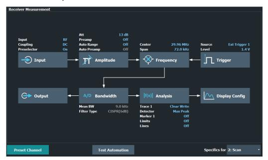
In addition to the main measurement settings, the configuration overview provides quick access to the main settings dialog boxes. Thus, you can easily configure an entire measurement channel from input over processing to output and analysis by stepping through the dialog boxes as indicated in the "Overview".
