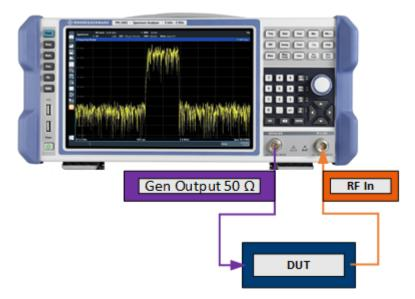
Figure 10-1: Test setup using the internal generator
