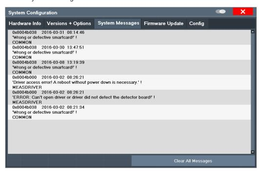
If the number of error messages exceeds the capacity of the error buffer, "Message Buffer Overflow" is displayed. To clear the message buffer, use the "Clear All Messages" button.
