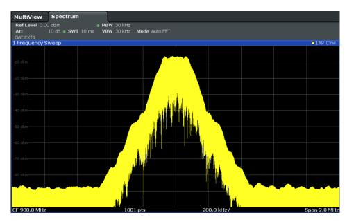
Figure 10-7: GSM signal with GATE ON
