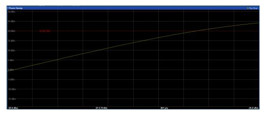
Thus, you can use the internal generator signal as a reference input signal for your power-converting DUT. Then you can compare the DUT input to its output at the RF input of the analyzer. Ideally, the result is a linear trace, that is: the output is directly proportional to the input power. Any distortion to the linear trace indicates the effects of the DUT. This result is useful, for example, to determine the compression point for amplifiers.
