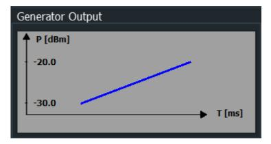
As a result, the measured power levels at the RF input are displayed versus the provided power levels of the internal generator output.
