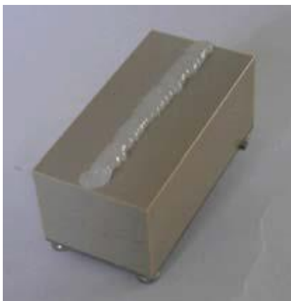
Figure 10 Applying ultrasonic couplant
