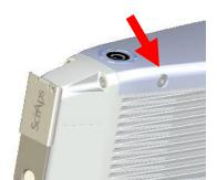
Press and hold the on/off button for 2 seconds.
