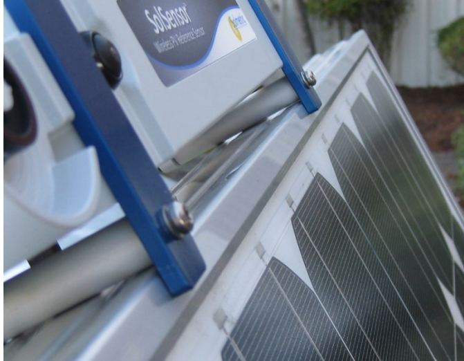
Figure 14. SolSensor correctly seated along the upper horizontal leg of the module frame.
