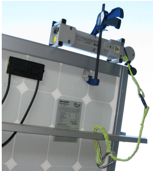
Figure 13. SolSensor tool lanyard secured to a racking member.
