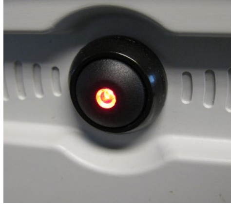
Figure 18. SolSensor pushbutton with LED lit. LED blinks until wireless network is established, after which it remains on.
