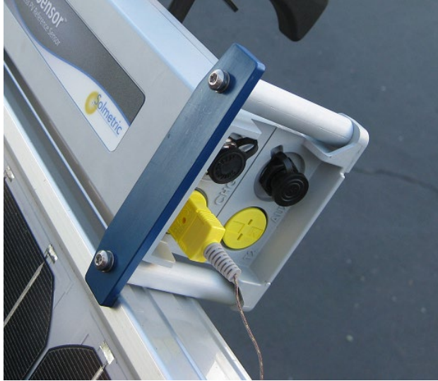
Figure 16. Thermocouple plugged into the TC1 connector.
