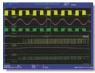
Measuring inverter I/O signals and control signals using the 10 MS/s high-speed 12-bit isolated module, current probe 700937 and isolated probe 700929
