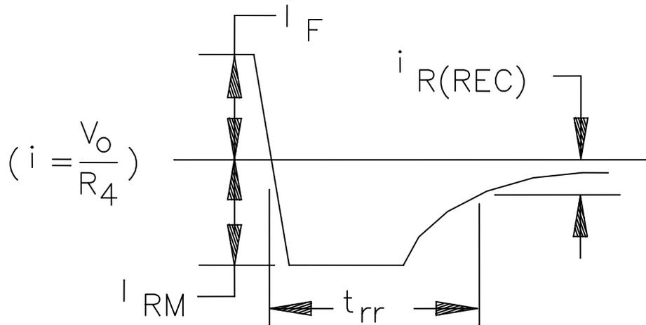
FIGURE 4031-5. Current through DUT (condition B).
