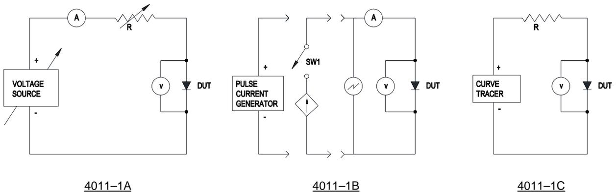
FIGURE 4011-1. Test circuits for forward voltage.
