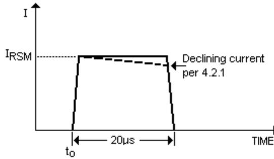
FIGURE 4065-2. Rectangular 20 μs Current Pulse Waveform.
