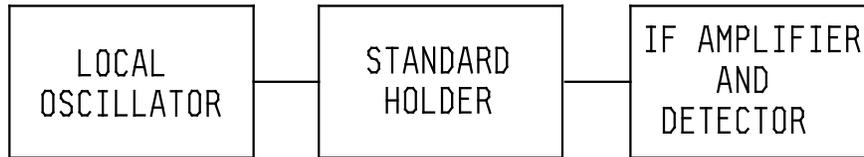
FIGURE 4121-1. Direct measurement method.
