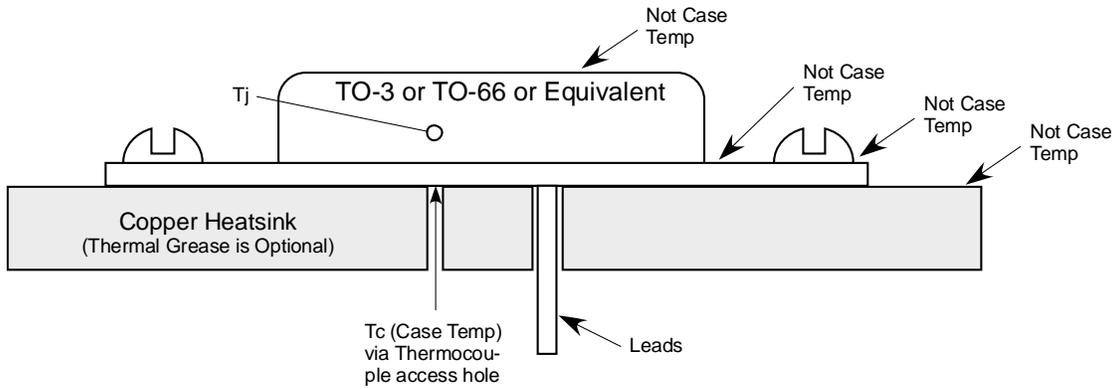
FIGURE 4081-4. Case mounting arrangement. (TO-3 or TO-66).
