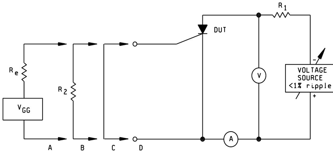
NOTE: The ammeter shall present essentially a short-circuit to the terminals between which the current is being measured or the readings shall be corrected for the drop across the ammeter.
