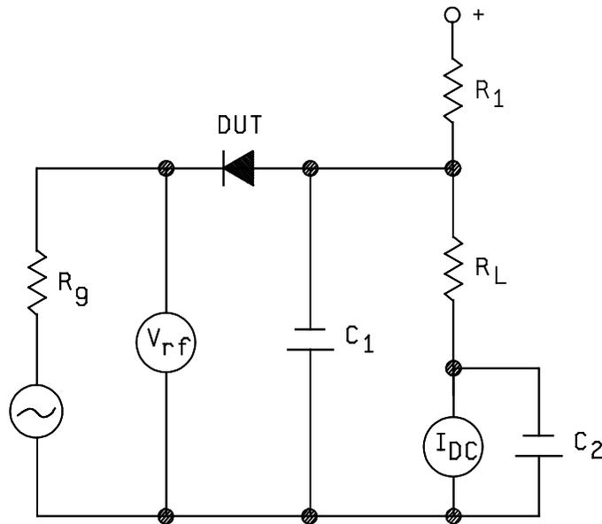
FIGURE 4106-1. Test circuit for detector power efficiency.
