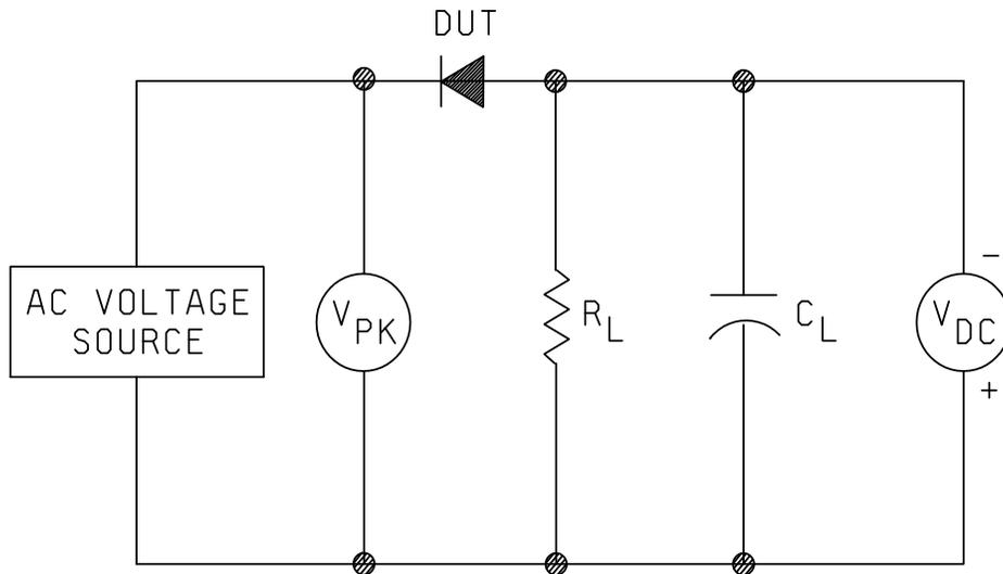
NOTE: The voltmeter shall have a high impedance as compared with the load circuit of  $R_L$  and  $C_L$ .
