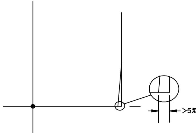
For standard rectifiers and zeners, the region at the knee may display a secondary trace no more than 5 percent of the total voltage of the DUT (see detail).
