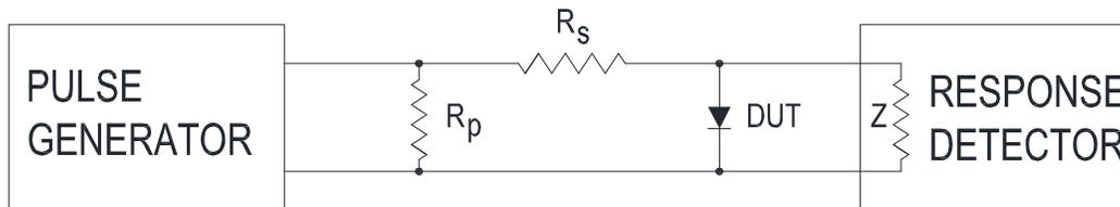
FIGURE 4026-1. Test circuit for forward recovery time and peak forward recovery voltage.
