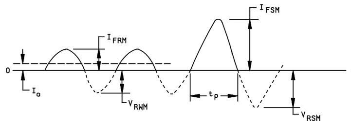
NOTE: Surge current pulse ( $t_p$ ) does not require synchronization with applied baseline ac.
