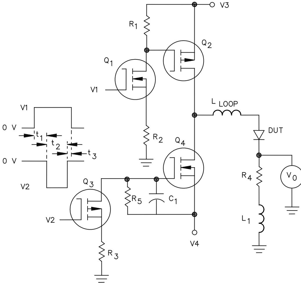
$V_1$  amplitude controls forward current ( $I_F$ ).
