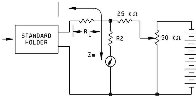
FIGURE 4101-2. Output circuit for the incremental measurement.
