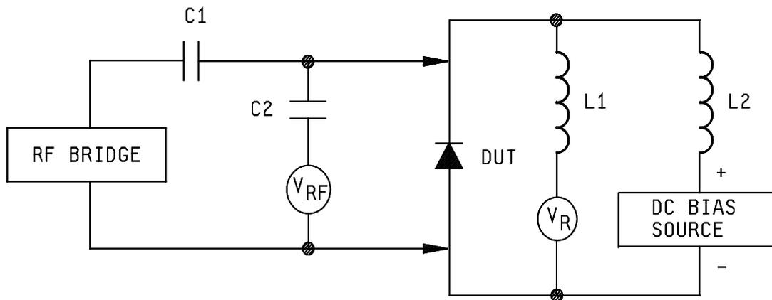
NOTE: The impedance of C1, C2, and L1, L2 shall be small and large, respectively, compared to the DUT at the frequency of measurement.
