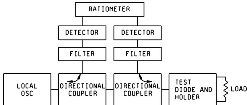
FIGURE 4136-2. Reflectometer method.
