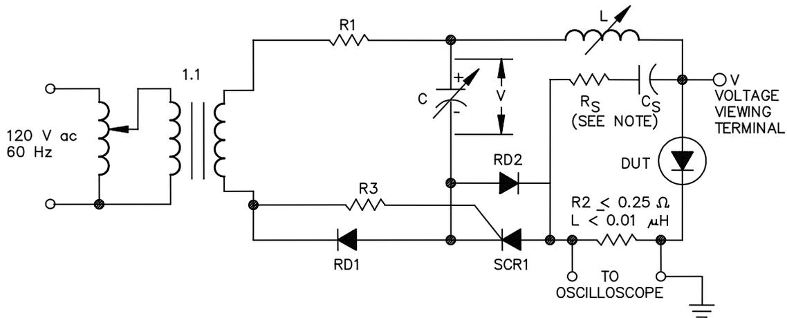
NOTE:  $R_s$  and  $C_s$  are snubber components, when their use is specified
