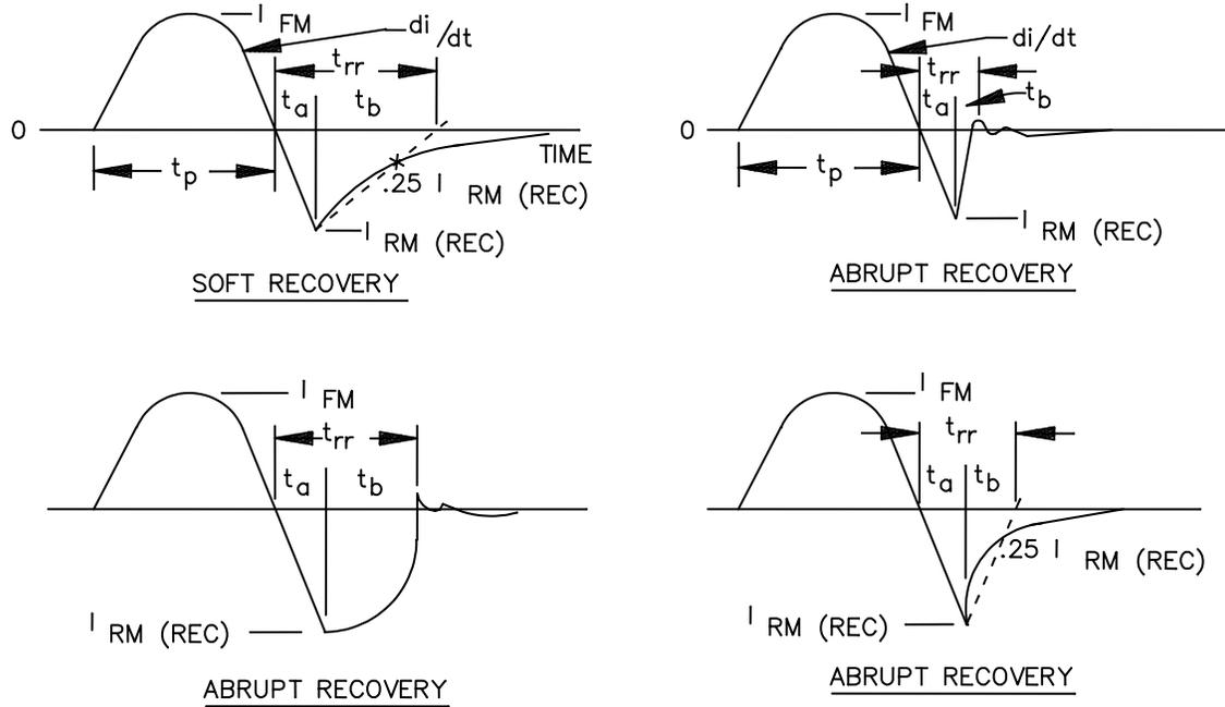
FIGURE 4031-7. Test current waveforms for various types of rectifier diodes under test in the circuit for measuring reverse recovery characteristics.
