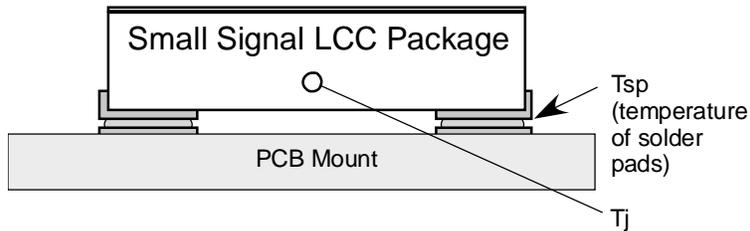
FIGURE 4081-6. Surface-Mount arrangement and Temperature Sensing Location (LCC).
