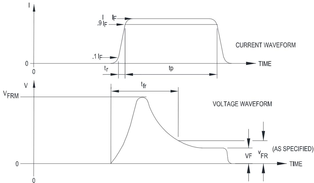
FIGURE 4026-2. Input forward current pulse and output voltage waveforms.
