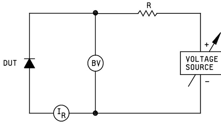
NOTE: The ammeter shall present essentially a short-circuit to the terminals between which the current is being measured or the voltmeter readings shall be corrected for the drop across the ammeter.
