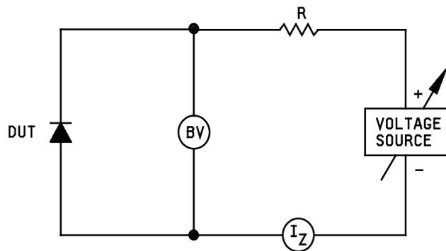
NOTE: The voltmeter being used to measure the terminal voltage should present an open circuit to the terminals across which the voltage is being measured.
