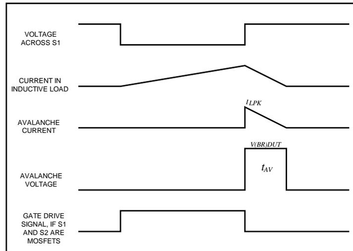
FIGURE 4064-4. Test Circuit 2 response.
