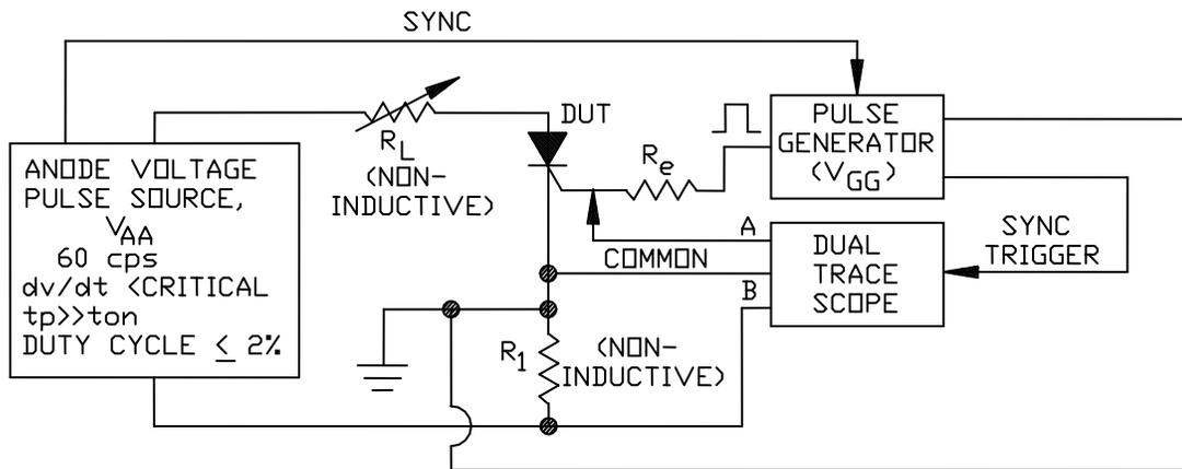
FIGURE 4223-1. Test circuit for gate-controlled turn-on time.
