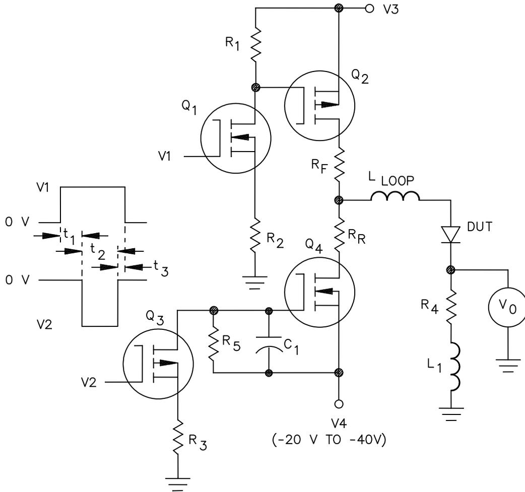
V<sub>3</sub> and R<sub>F</sub> control forward current I<sub>F</sub>
