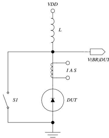
FIGURE 4064-1. Test circuit 1.
