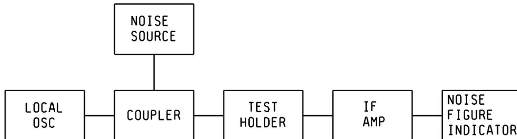
FIGURE 4126-1. Test setup for overall noise figure.
