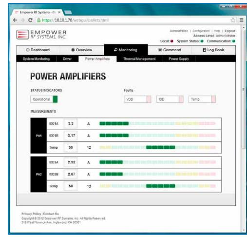
Integral to the performance of the overall HPA, **Power Amplifiers** display provides operating conditions and "wellness" for each of the RF output pallets. Color coded status for operating conditions and fault indicators provide additional visual feedback to the user.
