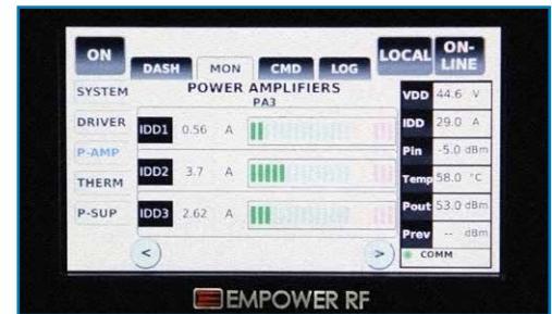
Notice the left side navigation where further drilling down of internal system functions can be viewed. This level of monitoring is a world's first providing the system engineer with a debug capability that quickly tells you if the system issues are up or downstream of the amplifier.
