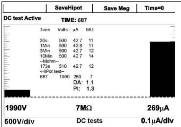
DC HiPot testing detects faults in groundwall/earth insulation, and also provides a complete Polarization Index test. The groundwall/earth insulation system consists of the wires insulation, slot liner insulation, wedges, varnish, and sometimes phase paper.
