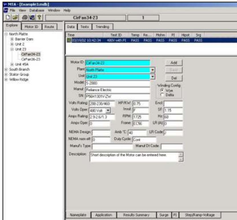
The Digital Winding Tester can operate on its own in the field, and then transfer the test data to a computer running Baker Instrument Company, an SKF Group Company's Motor Test Acquisition (MTA for Windows) software for further analysis. MTA for Windows provides database capabilities, waveform comparison, report generation, printouts, and other functions that turns test data into usable information. All options are easily accessed with on-screen prompts.
