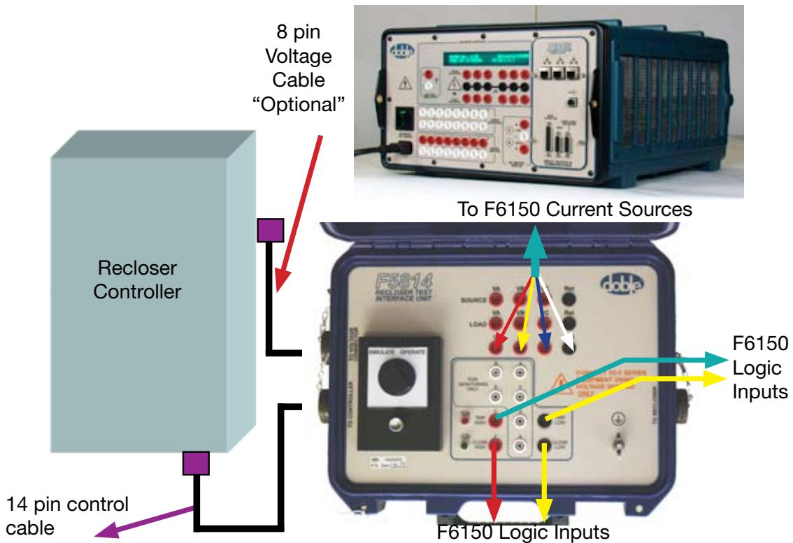
In this mode, the recloser is out of the circuit and hence the trip and close coils which are located in the recloser have to be simulated and this simulation is performed in the F5814. These simulated coils located in the F5814 react to the 24 Vdc that is provided by the recloser controller via the 14 pin control cable.
