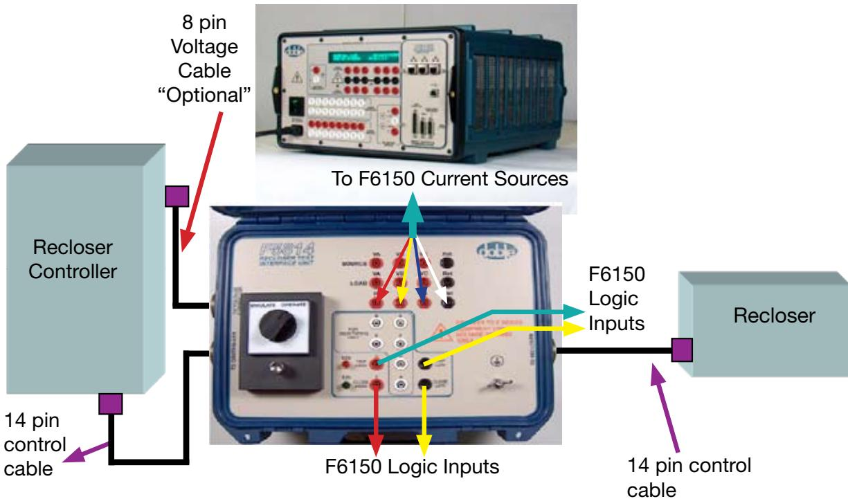
In this mode the simulated trip and close coils in the F5814 are bypassed and the F5814 simply passes the signal that it receives from the controller to the recloser trip and close coils. However, it still registers the trip and close status and passes this information to the F6150. The testing regimen conducted in the OPERATE mode are similar to the SIMULATE mode.
