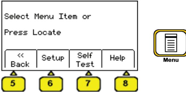
6. **Setup**: Displays second and third level screens for receiver configuration
