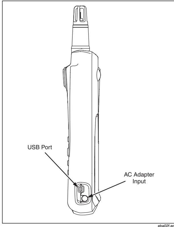
Figure 3. AC Adapter Input and USB Port
