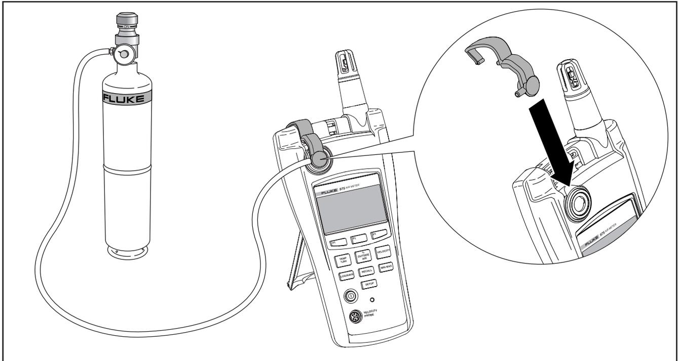
**Figure 4. Calibration Set Up**
