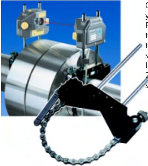
Quite possibly the only bracket you'll ever need: the standard ROTALIGN® PRO compact chain-type bracket ALI 2.891set uses interchangeable parts to fit onto shafts and solid couplings ranging from 15 mm to 500 mm (5/8" to 20") in diameter in a matter of seconds!
