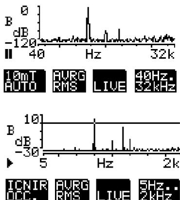
The EFA-300 is so powerful that even transient events ranging up to 2 kHz can be analyzed in real time.
