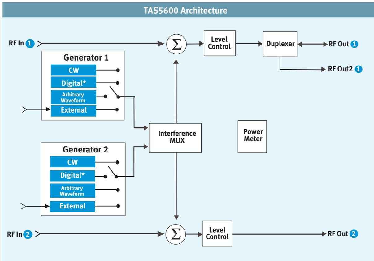
*TAS5600 combines precision interference generators, a power meter, attenuators, signal combiners and a duplexer in one compact, easy-to-control instrument.*
