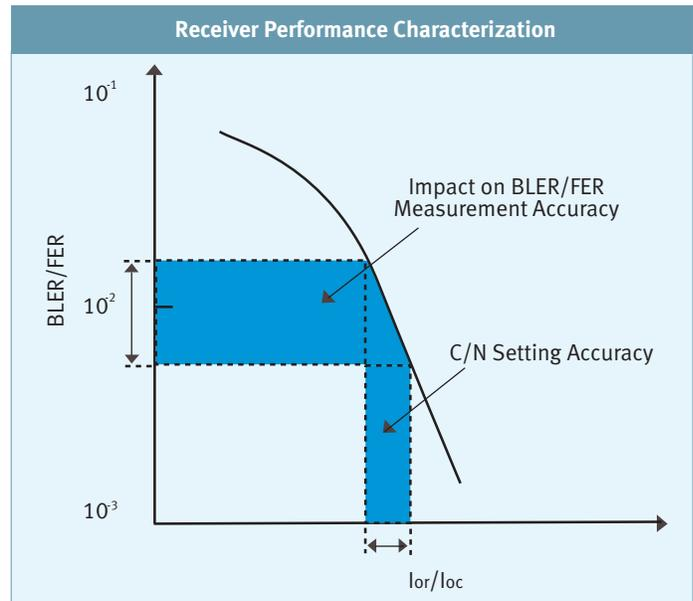
*TAS5600's high C/N (and C/I) ratio setting accuracy make it ideal for receiver performance breakpoint characterization.*
