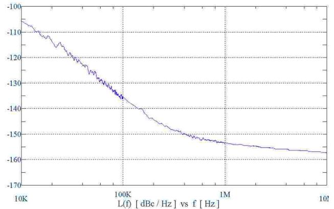
*TAS5600 with the Low Phase Noise Option demonstrates extremely low phase noise, eliminating co-channel noise during adjacent channel testing scenarios.*
