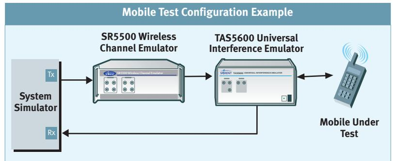
*TAS5600 and SR5500 combine to form a physical layer test system for base stations.*
