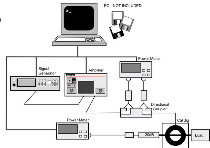
through which the cabling of the EUT is passed. Immunity tests are carried out by varying the test severity level and frequency of the induced disturbance. (ISO 11452-4 sect 4.1)
