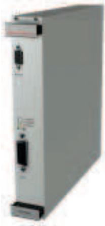
The controller controls all the addressing, real-time and synchronisation tasks on the CAN-bus as well as maintaining communication with the PC and, hence, with the AUTOSTAR user-software. RS 232C and IEEE 488 interfaces are available as standard. Designed as a motherboard, the unit can have other interfaces added as required. As a further facility, line
