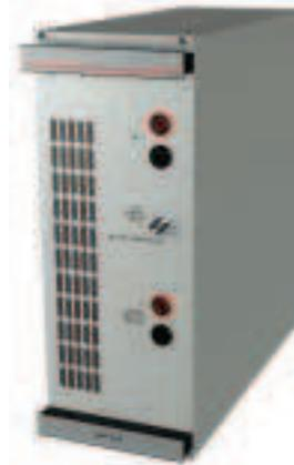
Up to ±15V and 5A can be delivered by the power amplifier module which means that for many applications – namely for component and sub-assembly testing – the use of an external battery simulator is unnecessary. The frequency range and bipolarity ensure that the module will find a wide range of applications. The EUT current can be
