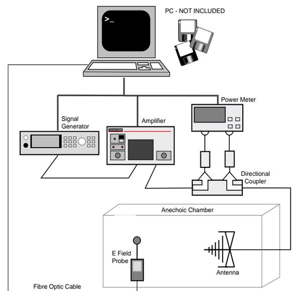
radiating the specified field strengths at the EUT with the available power may be used. (ISO 11452 sect 4.2.1)
