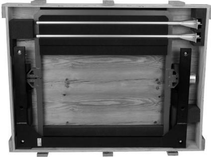
Unpack carefully the various parts. Check the parts for signs of transport damage. Any damage should be reported to the transportation company immediately.
