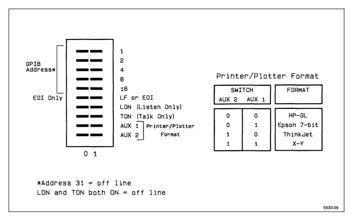
Figure B-16. Option 10 GPIB Interface PARAMETERS switch.
