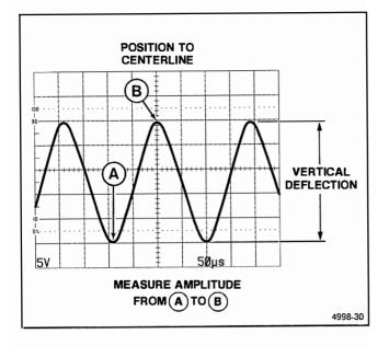
Figure 6-17. Peak-to-peak waveform voltage.
