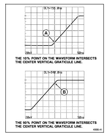
Figure 6-28. Rise time, differential time method.
