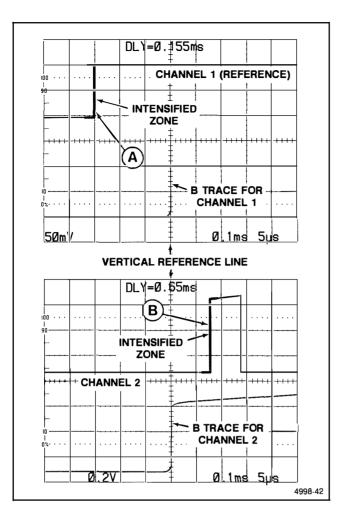
Figure 6-29. Time difference between two time-related pulses, differential time method.
