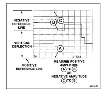
Figure 6-18. Ground referenced voltage measurement.
