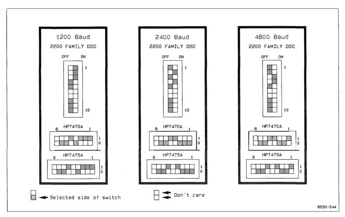
Figure B-11. Option 12 PARAMETERS switch settings for HP-GL compatible plotters.
