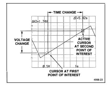
Figure 6-10. Slope using cursors.
