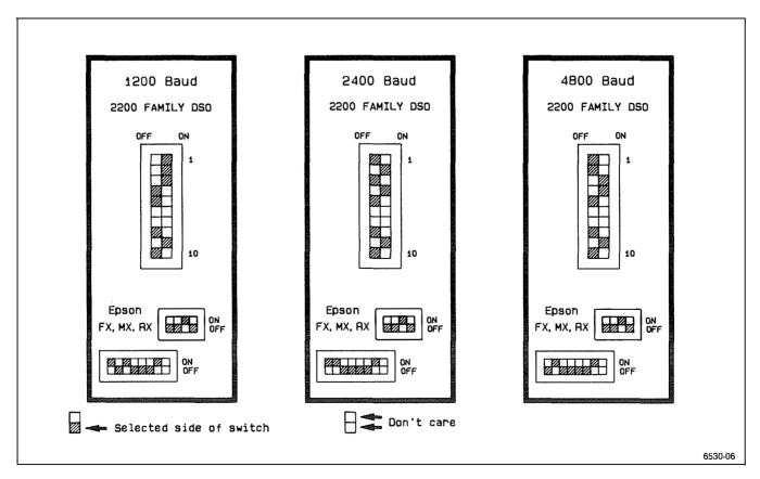
Figure B-13. Option 12 PARAMETERS switch settings for Epson printers.
