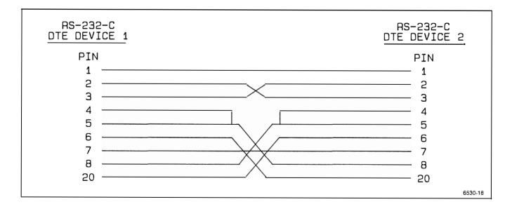
Figure B-1. Null Modem cable wiring (non-handshaking).
