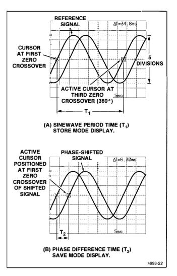
Figure 6-9. Phase difference between sinusoidal signals.
