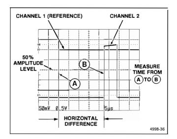
Figure 6-23. Time difference between two time-related pulses.
