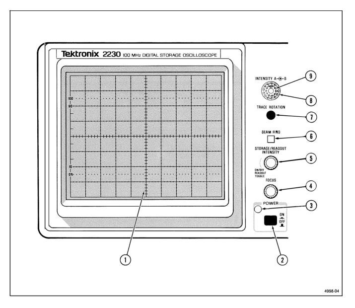
Figure 3-1. Power and display controls and power-on indicator.
