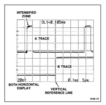
Figure 6-27. Time difference between repetitive pulses.
