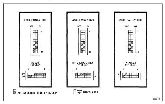
Figure B-17. Option 10 PARAMETERS switch settings for compatible GPIB printers/plotters.
