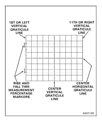
Figure 4-1. Graticule measurement markings.
