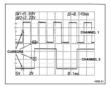
Figure 6-8. Time difference between two time-related pulses.
