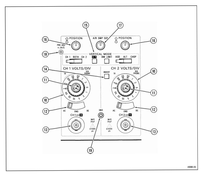
Figure 3-2. Vertical controls and connectors.
