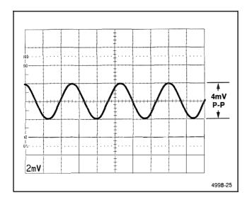
Figure 6-12. Low-level signal, AVERAGE mode.
