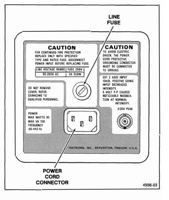
Figure 2-3. Fuse holder and detachable power-cord connector.
