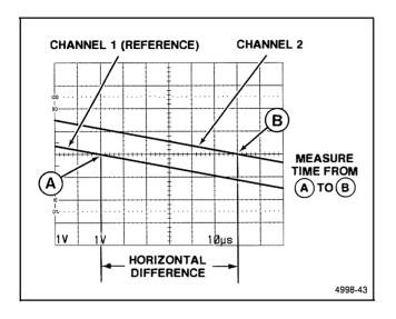
Figure 6-25. High-resolution phase difference.
