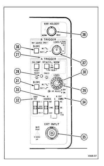
Figure 3-4. Trigger controls, connector, and indicator.
