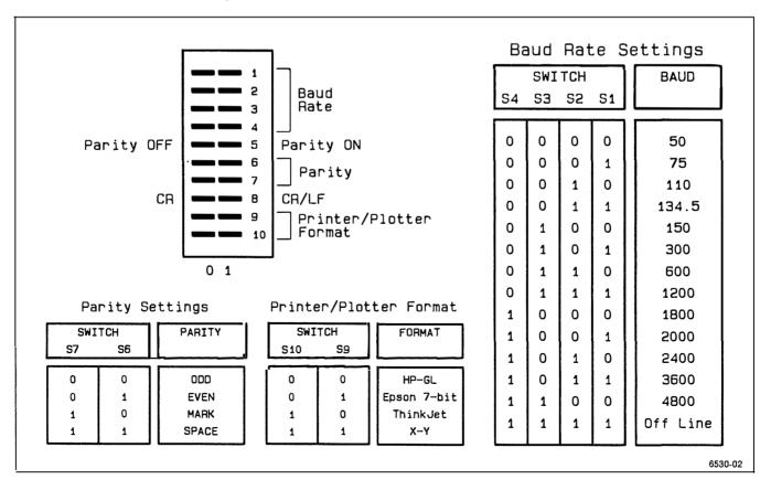
Figure B-9. Option 12 RS-232-C communication parameters.
