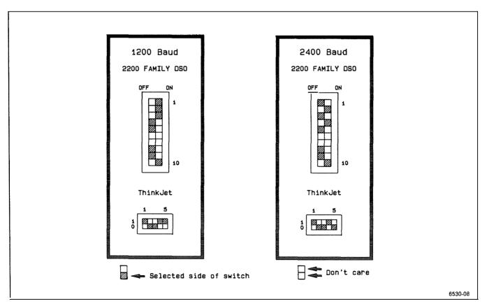
Figure B-15. Option 12 PARAMETERS switch settings for HP ThinkJet printer.
