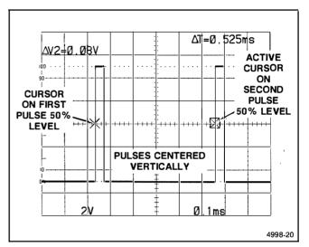
Figure 6-7. Time difference between repetitive pulses.
