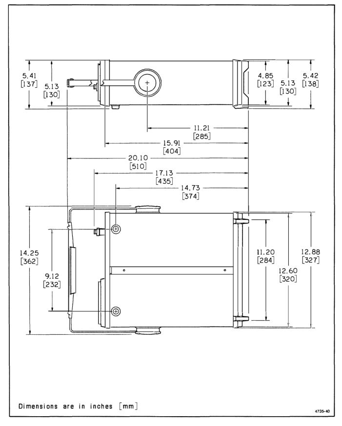
Figure 1-2. Physical dimensions of the 2230 Oscilloscope.
