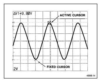
Figure 6-1. Ac peak-to-peak voltage, cursor method.
