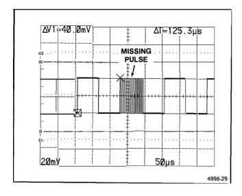
Figure 6-16. Missing pulse, ACCPEAK STORE mode.
