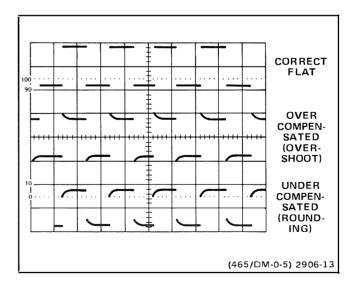
Figure 5-1. Probe compensation.
