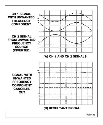
Figure 6-20. Common-mode rejection.
