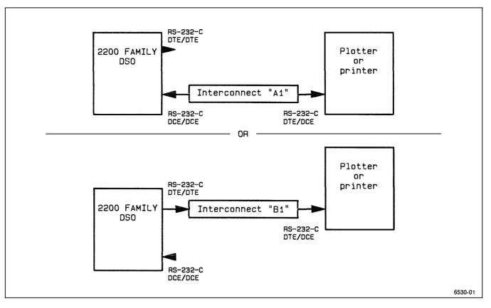
Figure B-8. Option 12 RS-232-C Printer/Plotter interconnects.
