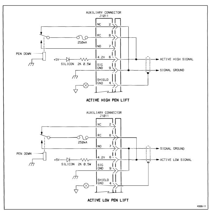
Figure 3-8. X-Y Plotter interfacing.
