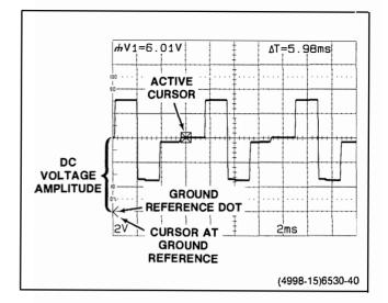
Figure 6-2. Ground referenced dc voltage, cursor method.
