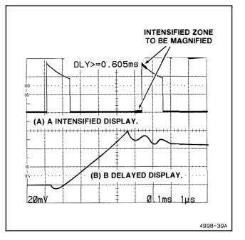
Figure 6-26. Delayed-sweep magnification.
