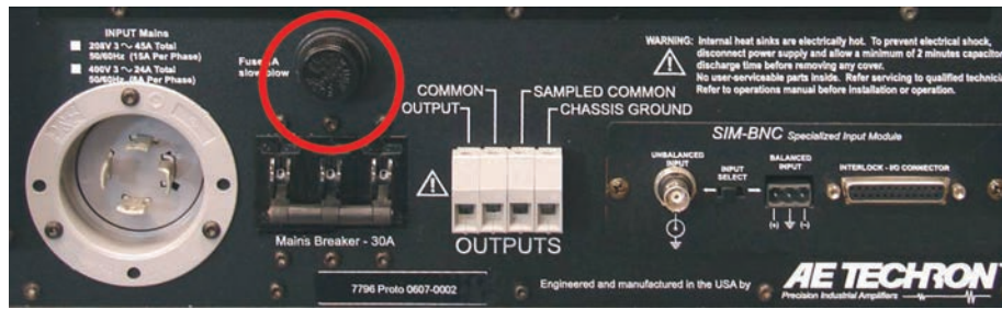
Figure 7.3 – Fuse F1 Location
