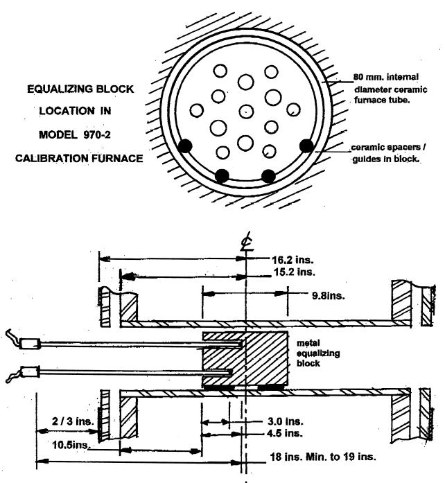
INSERTION DEPTH & EQUALIZING BLOCK POSITION -- "STANDARD" PROBES
