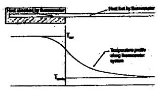
FIG. 1: The flow of heat down the stem of a thermometer causes the thermometer to indicate temperatures lower than the medium of interest.
